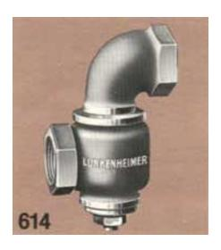
Swing joints are most frequently used on machine tools in the cutting-fluid lines. The rate of flow through the line is usually controlled by a cock.
